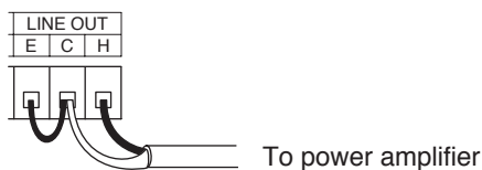
[Connection to an unbalanced amplifier]
